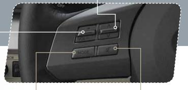
Press the button to select the desired audio mode – FM, AM, SAT, CD, AUX, MEDIA.
